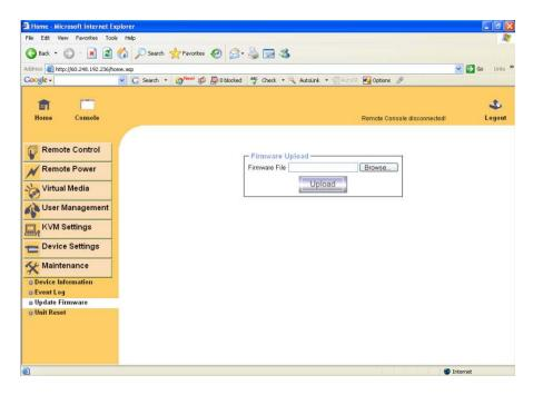
The IP module is a complete standalone computer. The software it runs is called firmware. The firmware of the IP module can be updated remotely in order to install new functionality or special features.
