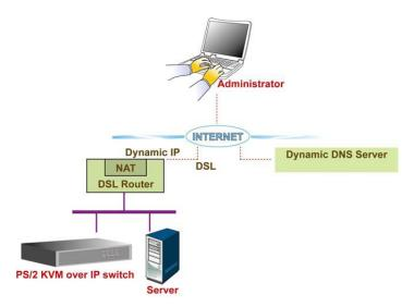
The IP module is reachable via the IP address of the DSL router, which is dynamically assigned by the provider. Since the administrator does not know the IP address assigned by the provider, the IP module connects to a special dynamic DNS server in regular intervals and registers its IP address there. The administrator may contact this server as well and pick up the same IP address belonging to his card.
