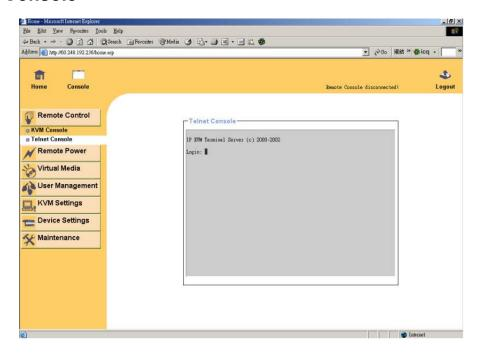
The IP module firmware features a Telnet server that enables a user to connect via a standard Telnet client. In case the Telnet program is using a VT 100, VT 102 or VT 220 terminal or an according emulation, it is even possible to perform a console redirection as long as the IP module host machine is using a text mode screen resolution.
