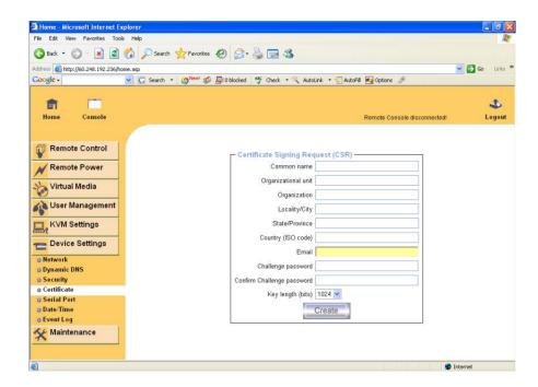
The IP module uses the Secure Socket Layer (SSL) protocol for any encrypted network traffic between itself and a connected client. During the connection establishment the IP module has to expose its identity to a client using a cryptographic certificate. The default certificate comes with IP MODULE device upon delivery is for testing purpose only. System administrator should not rely on this default certificate as the secured global access mechanism through Internet.
