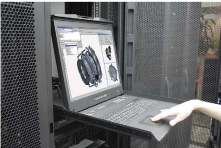
Figure 6. Operating the LCD keyboard drawer
