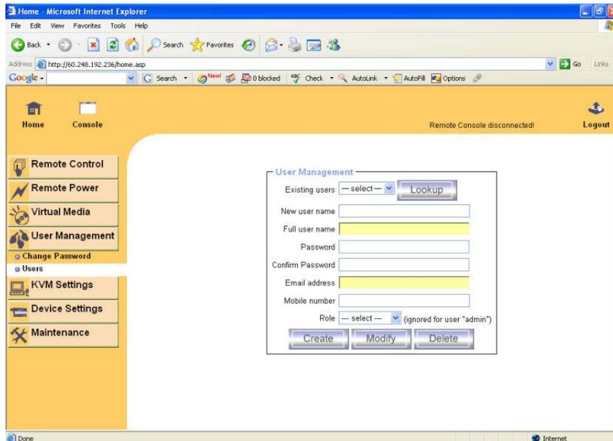
The IP module comes with 1 pre-configured user account that has fixed permissions. The account “super” has all possible rights to configure the device and to use all functions IP module offers.
