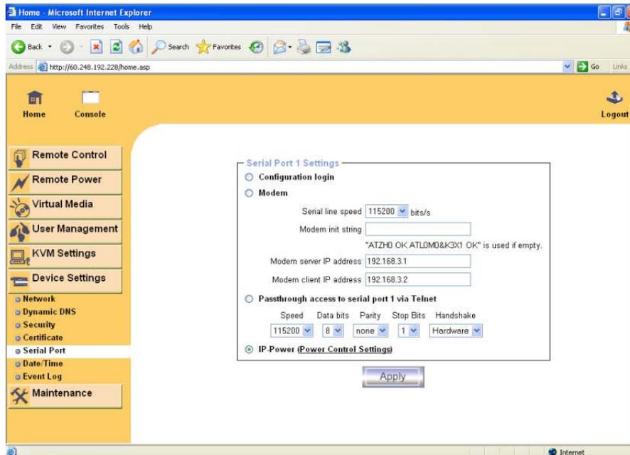
The IP module Serial Settings allows you to specify what device is connected to the serial port and how to use it.
