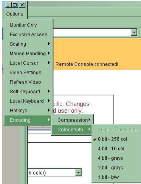
**Note:** If displaying motion pictures on a connection with low speed you may achieve an improvement regarding the video transfer rate by lowering the color depth and disabling the option “Video Optimized”. As a general result, the data rate is reduced (less bits per color). Furthermore, the OPMA module will not have to do any video compression. In total, this will lead to less transfer time of the motion picture.
