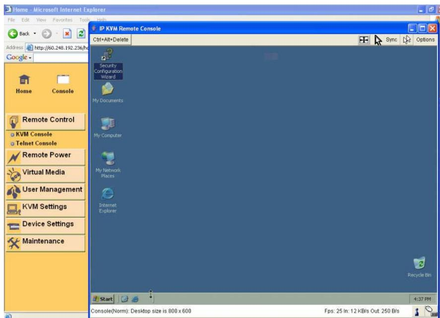
To open the KVM console, either click on the menu entry on the left, or on the console picture on the right. To refresh the picture, click on the button “Refresh”.
