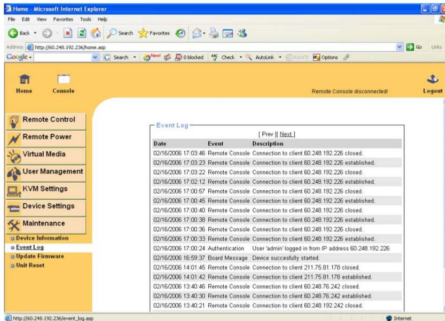
The image above displays the log list including the events that are logged by the IP module.
