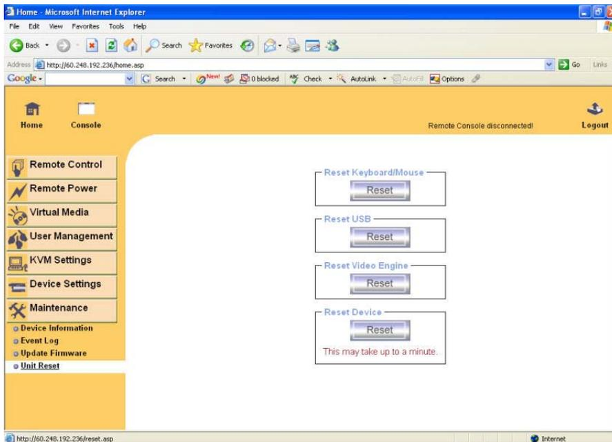
This section allows you to reset specific parts of the device. This involves the both keyboard and mouse, the video engine and the IP module itself. Resetting the card itself is mainly needed to activate a newly updated firmware. It will close all current connections to the administration console and to the Remote Console.
