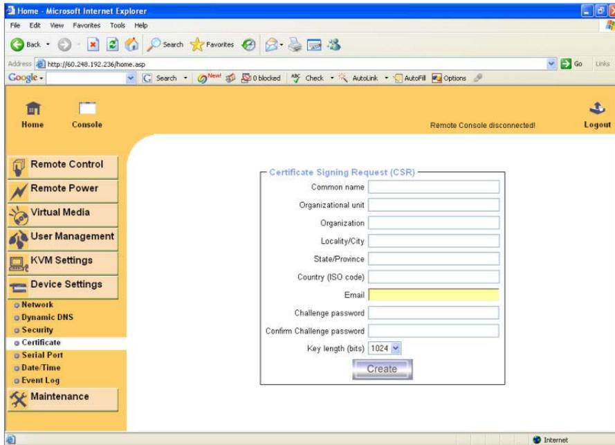
The IP module uses the Secure Socket Layer (SSL) protocol for any encrypted network traffic between itself and a connected client. During the connection establishment the IP module has to expose its identity to a client using a cryptographic certificate. The default certificate comes with IP MODULE device upon delivery is for testing purpose only. System administrator should not rely on this default certificate as the secured global access mechanism through Internet.
