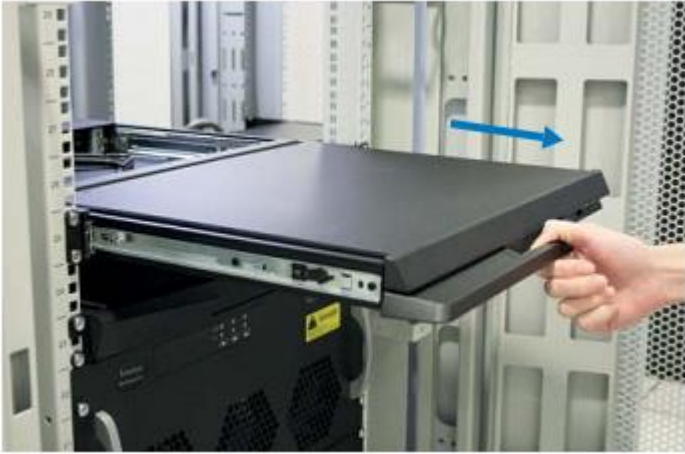
Figure 4. Sliding out the LCD keyboard drawer by pulling the tab toward the front of LCD.
